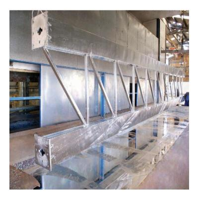
**A 153/A 153M.** Standard Specification for Zinc Coating (Hot-Dip) on Iron and Steel Hardware
