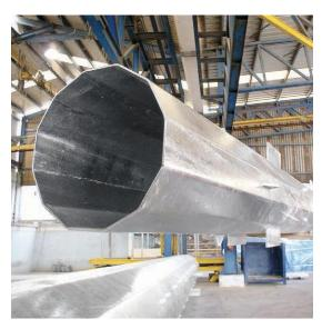
This process is carried out through immersion of materials into a bath of molten zinc. Due to the fact that the pieces are totally immersed in the liquid metal, the surface is completely covered and protected from possible corrosive effects which could be caused by the atmosphere, water or surface.
